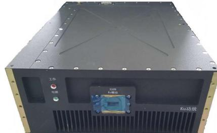
Ku band 400W solid state power amplifier can be used in satellite communications, data link and measurement and control
